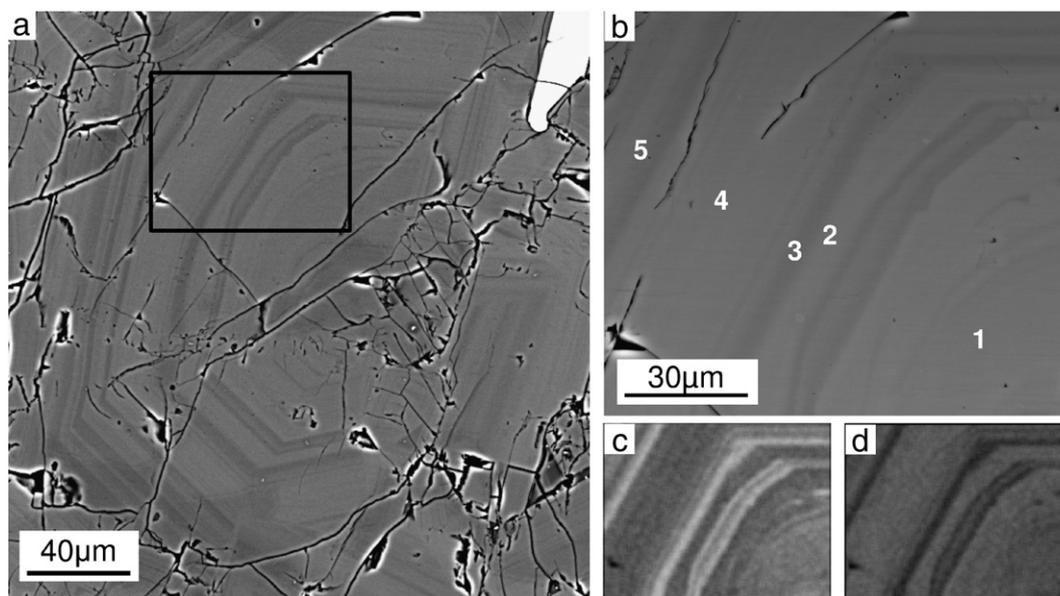
**Fig. 7.** BE image corresponding to crystal 1 (a), and the detailed zone chosen for XRM acquisition (b). Na and Ca XRMs from the selected area (c and d).
