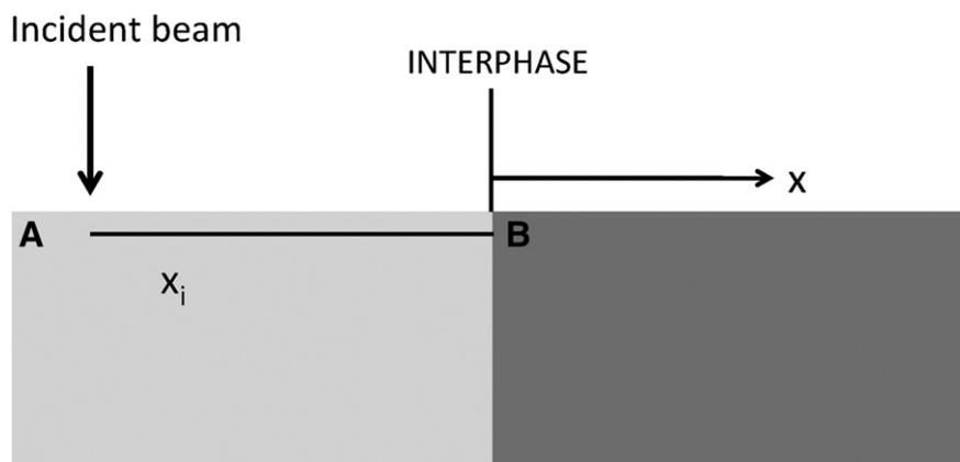
Fig. 1. Settings used to study the spatial resolution for sodium and calcium characteristic X-rays, as well as the interface crossing effect in the BE signal near the interface A|B defined by the A (left) and B (right) materials.
