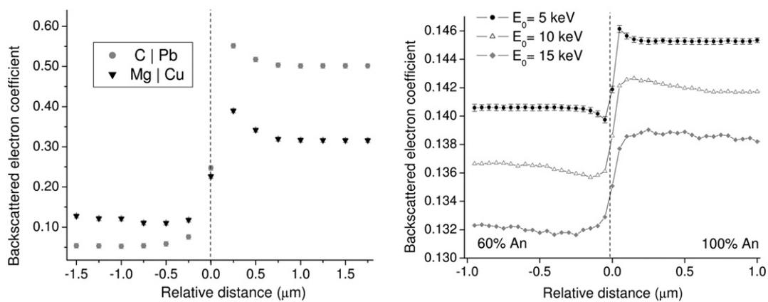
**Fig. 6.** Monte Carlo simulations for the backscattered electron distribution as a function of the distance relative to the interface for Mg|Cu, C|Pb irradiated at 20 keV (right) and An 60%|An 100% irradiated at 5, 10, and 15 keV (left).
