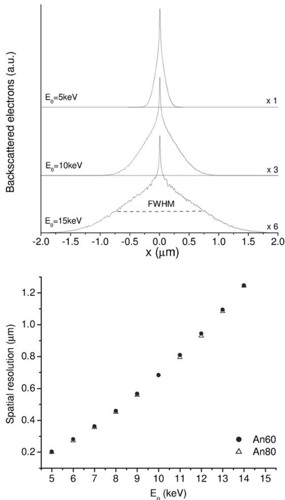
**Fig. 2.** Results of Monte Carlo simulations for the backscattered electron spatial distribution in a labradorite plagioclase (An 60%) around the electron impact point at 5, 10 and 15 keV (top). Spatial resolution for BE signal in An 60% and An 80% (bottom).
