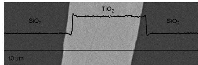
Fig. 4. Experimental gray level variation along a profile corresponding to a rutilitated quartz sample, measured at 15 keV.
