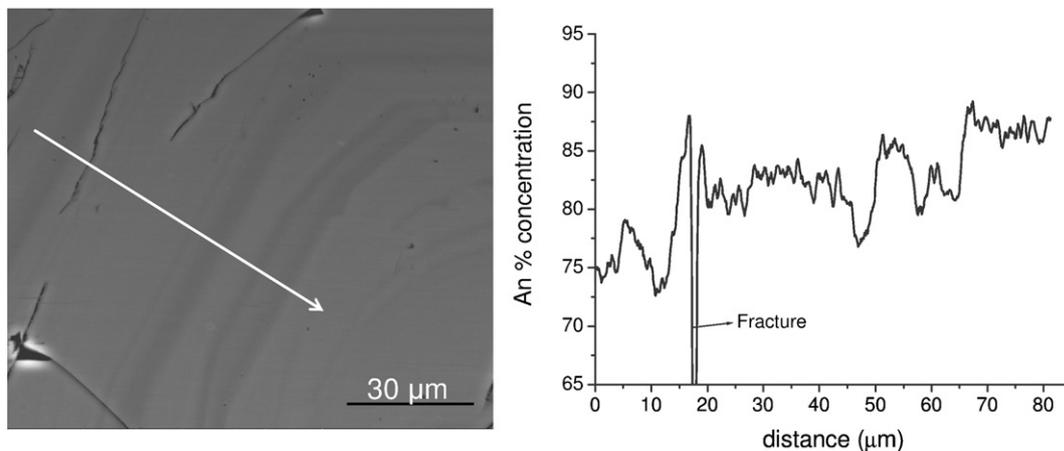
**Fig. 10.** Calibrated BE images (left) and quantitative An-calibrated gray-level profile in the indicated zones for the crystal 1.
