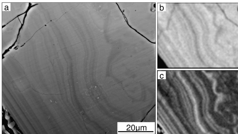
**Fig. 8.** BE image corresponding to crystal 2 (a) and the XRMs for Na and Ca taken in the selected area (b and c).
