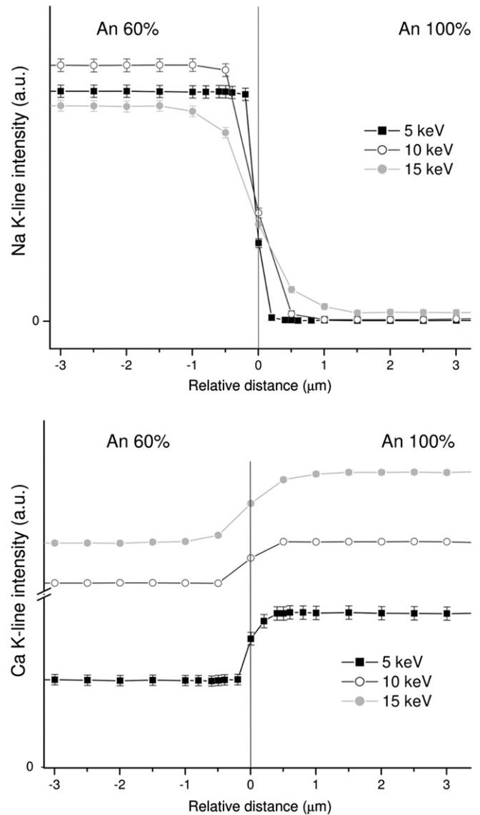
**Fig. 3.** Na (top) and Ca (bottom) X-ray intensities for a sample with an interface separating An 60%/An 100%, obtained by Monte Carlo simulation for incident energies of 5, 10 and 15 keV. Error bars correspond to statistical uncertainties inherent to the simulation routine.
