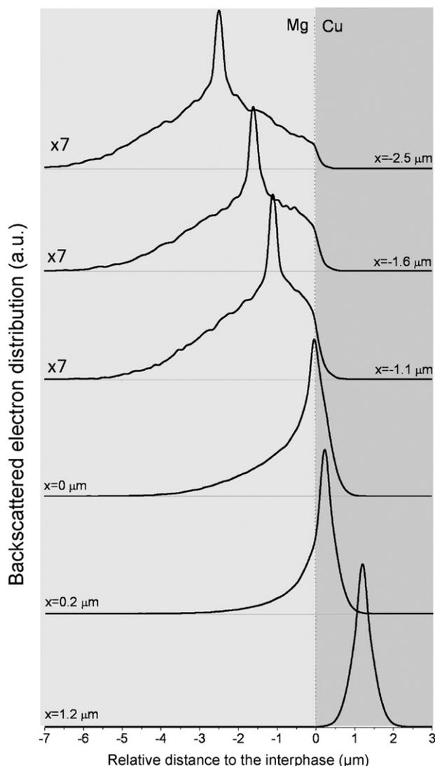
Fig. 5. Monte Carlo simulations for the lateral distribution of backscattered electrons at different distances  $x_i$  from the impact point, for a beam energy of 20 keV. The interface corresponds to a Mg|Cu system. The vertical scales in the first three plots were multiplied by 7 to help visualization.
