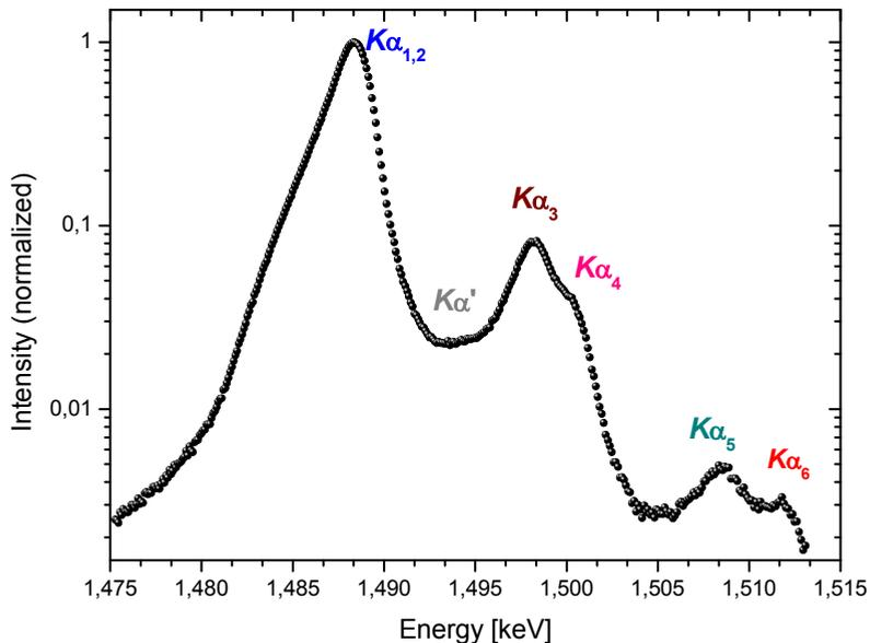
Fig. 5. Al  $K\alpha$  spectrum measured through XRF.
