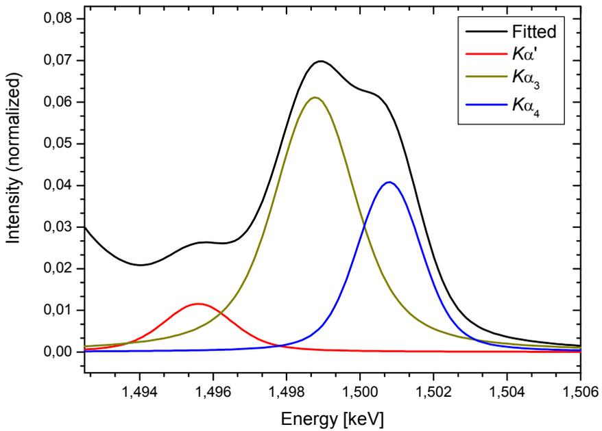
Fig. 10. Satellite lines measured in  $Al_2O_3$  with XRF.
