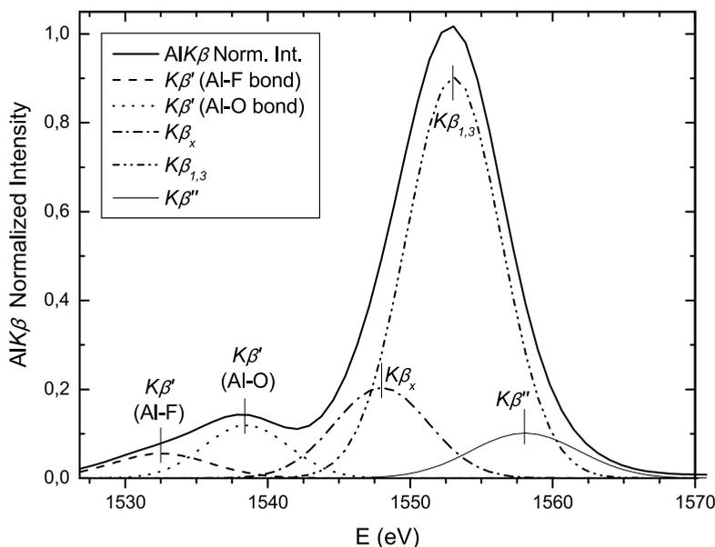
Fig. 11. Al  $K\beta$  spectrum of Topaz. The two  $K\beta'$  lines (due to the Al-F and Al-O covalent bonds) and the Al  $K\beta_x$ , Al  $K\beta_{1,3}$  and Al  $K\beta''$  lines have been deconvoluted with Gaussian functions and its energies are pointed out. The spectrum is normalized to the height at the maximum intensity point. (Torres Deluigi et al., 2006).
