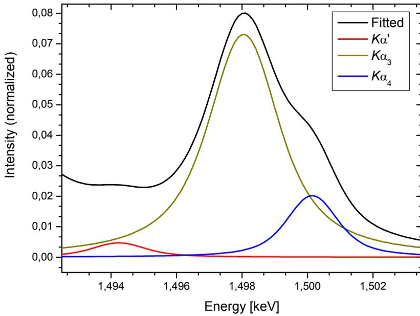
Fig. 9. Satellite lines measured in Al with XRF.
