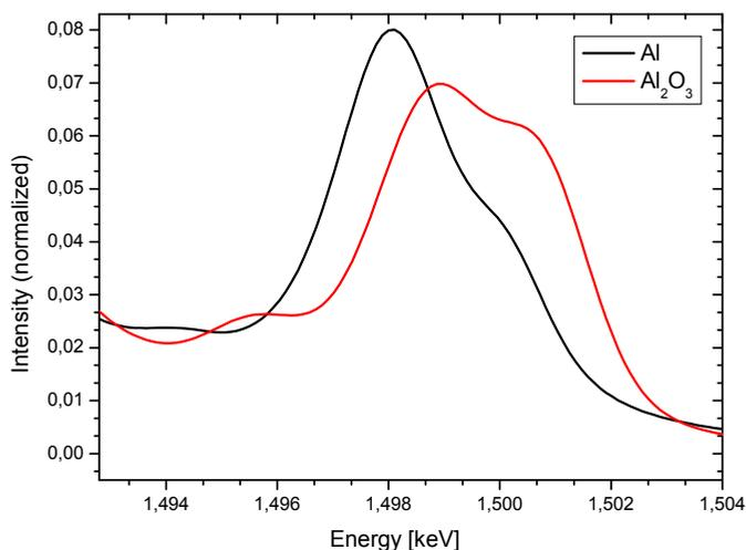
Fig. 8. Satellite spectra of Al and Al<sub>2</sub>O<sub>3</sub> measured through XRF.
